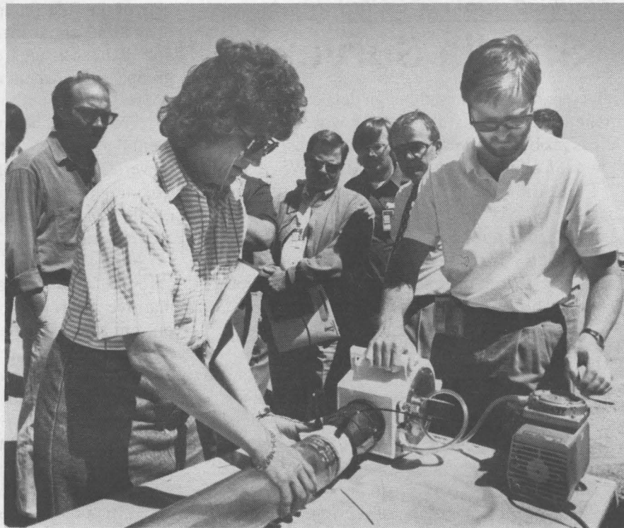
SAMPLING SOCK — Cecelia Williams (7721) and Dave Cremer (Science and Engineering Associates) demonstrate SEAMIST™ to a group of industry representatives May 25. SEAMIST, one of several environmental restoration technologies now under development at Sandia, is an inflatable membrane that can carry sampling instrumentation into boreholes to measure subsurface conditions such as soil moisture, soil content, etc. It also helps maintain borehole integrity. For more on SEAMIST, see the May 14 LAB NEWS.
